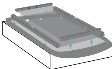
5. Place the foam support layer between the rails and smooth it out to fill the entire base.
