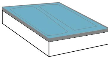
10. Place the comfort layer across the top of the air chambers and foam rails.
