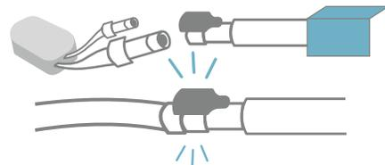
7. Connect the air control unit to a powered surge protector & plug the hand controls into the each side. The hand control will operate the air chamber on the side that it is plugged into.\*
