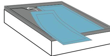
7. Connect the tubes from the air chambers to the connectors on the pump. Press the two ends together until you hear a "Click." Be sure to keep track of which hose connects to which side of the pump.
