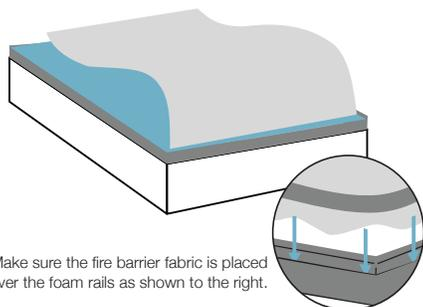
Make sure the fire barrier fabric is placed over the foam rails as shown to the right.
